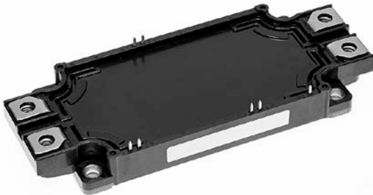
dual switch (Half-Bridge)
